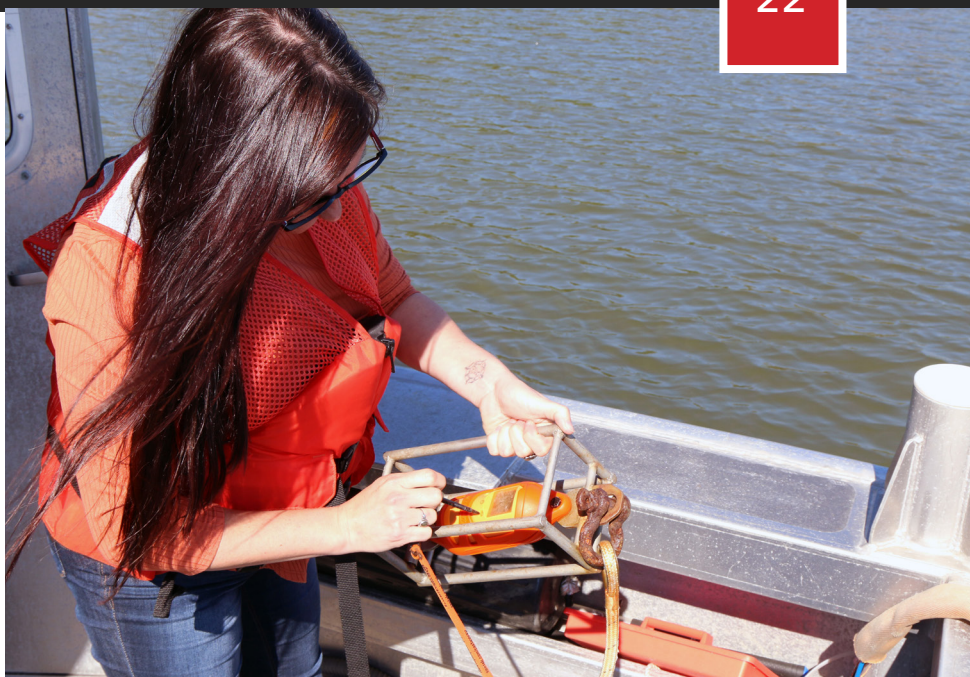
Sonja Zindars prepares to drop a Castaway CTD into the water. The device measures conductivity, temperature and depth to determine a speed of sound change throughout the water column.
